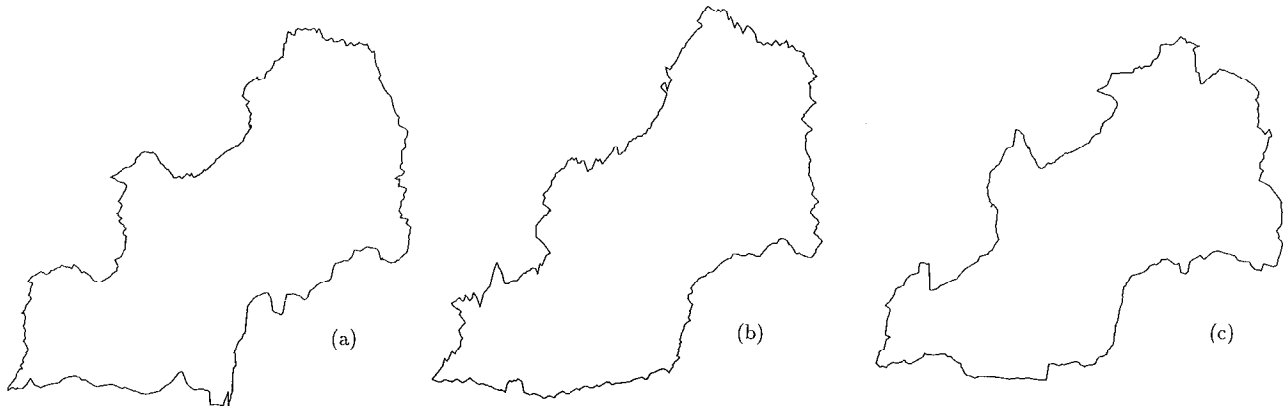
Figure 3. (a, b) Two realizations of the boundaries of the structure resulting from the procedure described here. The width function of the Nelk river basin is imposed and is exactly reproduced in all realizations; (c) the reconstructed shape as the ensemble average of 10 realizations of the shapes devised according to the approach described here.
